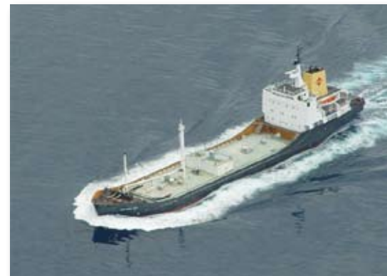
The M.V. Golden Bay: a cement carrier with a capacity of 4,500 tonnes.
