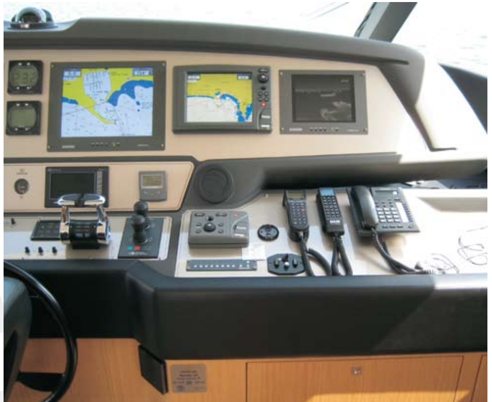
The joystick to control the FLIR Systems thermal imaging camera and the LCD display on which the thermal images are displayed are esthetically integrated in the bridge of the Ziacania
