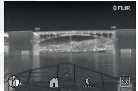
Thanks to small icons conveniently placed at the bottom of the thermal image, the captain can see immediately in which direction the Navigator is looking, whether it is in the "home position" or not. Also other settings of the camera can easily be read from these icons.
