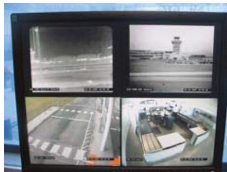
Top left and right: Images from the SR-100 thermal imaging cameras displayed on an LCD screen
