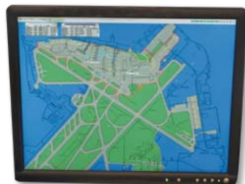
Ground radar follows everything leaving or entering the Critical part of the Security Restricted Area (CSRA). The borders of the CSRA are marked with a red line.
