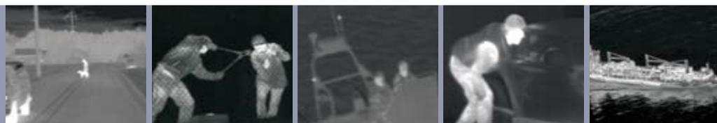
In contrast with other technologies, such as light amplification, thermal imaging needs no light whatsoever to produce an image on which the smallest of details can be seen. Thermal imaging provides full visibility irrespective of the prevailing light level and weather conditions. It can see in total darkness, through light fog, in the far distance, through smoke and is able to detect anyone hiding in the shadows. It is an excellent tool for security and surveillance applications in marinas.
