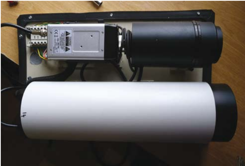
The FLIR Systems SR-100 thermal imaging camera (bottom) and a CCTV camera as they are mounted inside the stainless steel housing.
