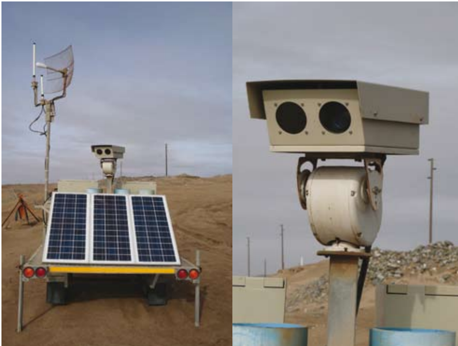
A moveable trailer with solar panel. The FLIR Systems SR-100 thermal imaging camera is mounted in a stainless steel protective housing which protects it against the harsh weather conditions alongside the Namibian coast.
